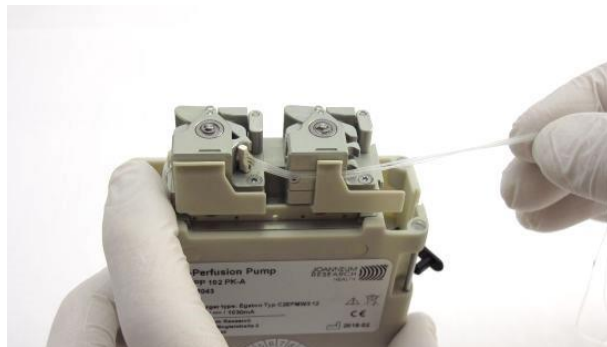
Figure 16a: Tubing is fixed with retaining springs in the pump.
