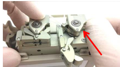
Figure 15: Inserting the tubing into the pump module
