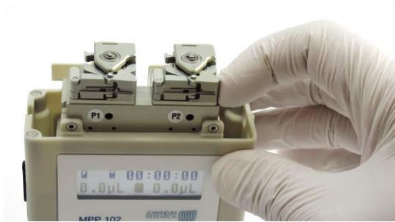
Figure 14: Opening of pump head using the snap mechanism.
