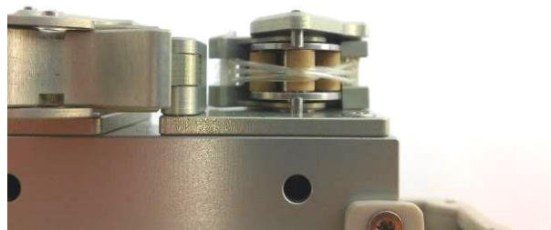
b: Tubing set inserted INCORRECTLY
