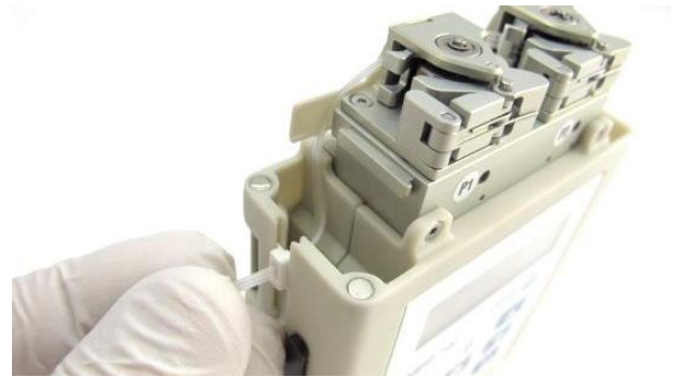
b: Tubing with strain relief is placed into the slot located on the left side of the pump.
